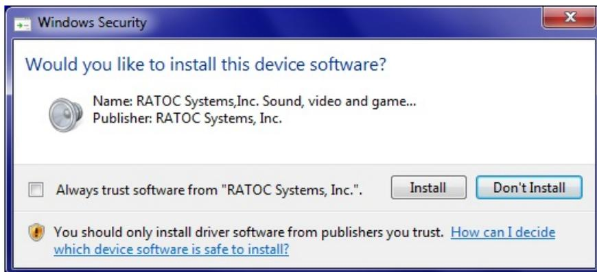
(9) When this message shows up, remove USB Audio Device except RAL-KEB02iP. Only one KEB02iP should be connected at this time. Click "OK", "Next", "Install", "Install" to finish the installation.
