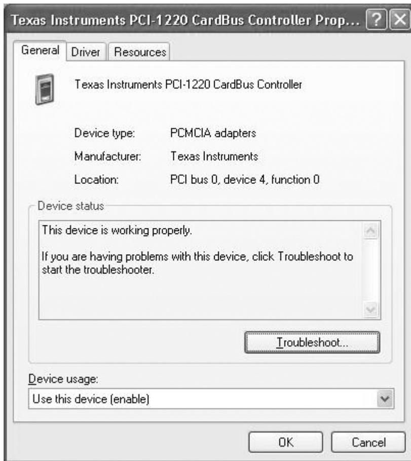
2. Grasp the CB31U by the edges with the label facing upward. Insert the CB31U into the slot and push it in until it is firmly seated. If the CB31U can not be firmly seated, check to see if the PC Card slot supports CardBus PC Cards. If the following windows do not appear, the PC may not support CardBus PC Cards. Check to see if the PC Card slot supports CardBus PC Cards. For more information, contact your PC manufacturer.
