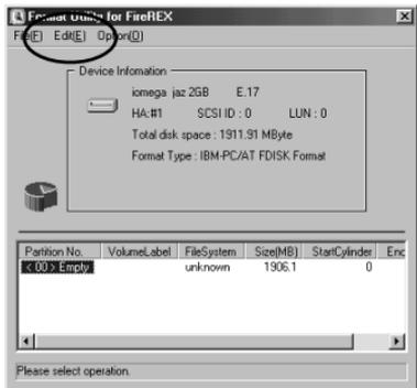
7. The Initialize/Format screen will appear. Select **format type**. If you want to do Low Level Format simultaneously, check **Low Level Format**. Then, click **OK**.
