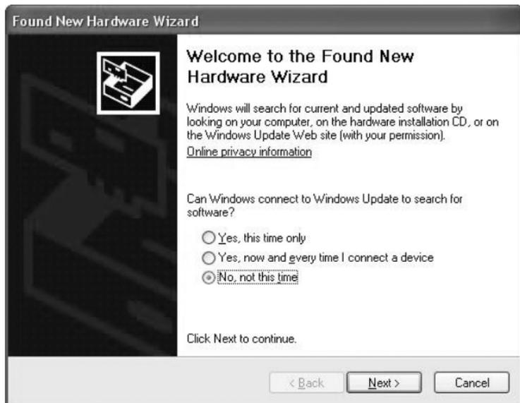
If the New Hardware Wizard doesn't appear, but there is a yellow '!' point on "RATOC System\_Inc. IEEE1394-SCSI-3 IEEE1394 SBP2 Device" on the **Device Manager**, the driver of the SCSI device needs to be installed. (To open the device manager: Go to "Start" - Right click on "My Computer" - Properties - Hardware - Device Manager button.)
