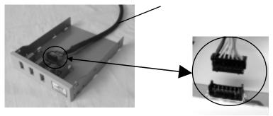
2. Insert the front-bay extension adapter into 3.5 inch bay, as shown below. Then, connect the front-bay extension adapter to 3.5 inch bay with the screws provided, as shown below.
