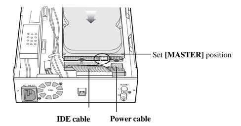
(7) Fix the drive to inner case by screws. Then, replace the top cover and slide back the inner case into enclosure. You have finished mounting a drive. Proceed to Chapter 2-2.
