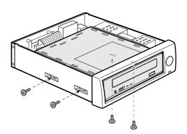
(6)If you mount a 3.5 inch hard drive, set [MASTER] position in jumper setting. Then, connect IDE cable, power cable.
