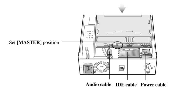
(5) Fix the drive to inner case by screws. Then, replace the top cover and slide back the inner case into enclosure. You have finished mounting a drive. Proceed to Chapter 2-2.
