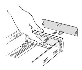
(4)Set [MASTER] position in jumper setting. Then, slide a 5 inch drive such as a CD-ROM into inner case and connect IDE cable, power cable and analog audio cable(red-colored line is R; white-colored line is L).
