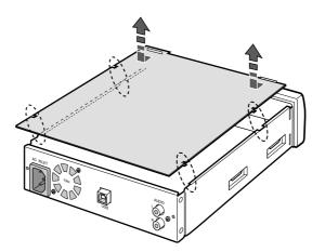
(3)Push the hook on front panel to release front cover if you mount a 5 inch drive. If not, you don't need to release it. In such a case, proceed to step (6).
